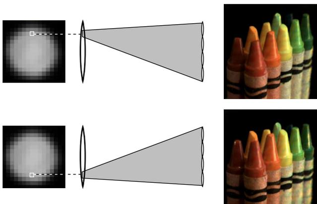
**Figure 4:** Two sub-aperture photographs obtained from a light field by extracting the shown pixel under each microlens (depicted on left). Note that the images are not the same, but exhibit vertical parallax.
