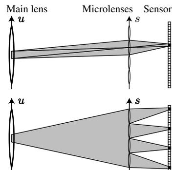
**Figure 3:** *Top:* All the light that passes through a pixel passes through its parent microlens and through its conjugate square (sub-aperture) on the main lens. *Bottom:* All rays passing through the sub-aperture are focused through corresponding pixels under different microlenses. These pixels form the photograph seen through this sub-aperture (see Figure 4).
