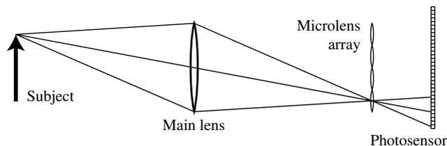
**Figure 1:** Conceptual schematic (not drawn to scale) of our camera, which is composed of a main lens, microlens array and a photosensor. The main lens focuses the subject onto the microlens array. The microlens array separates the converging rays into an image on the photosensor behind it.
