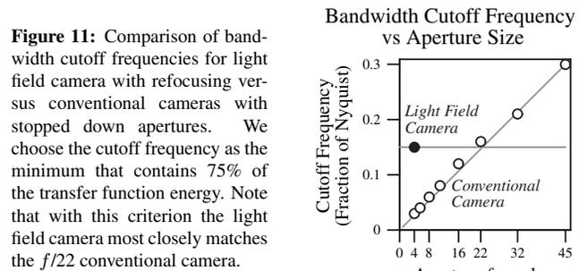
**Figure 11:** Comparison of bandwidth cutoff frequencies for light field camera with refocusing versus conventional cameras with stopped down apertures. We choose the cutoff frequency as the minimum that contains 75% of the transfer function energy. Note that with this criterion the light field camera most closely matches the  $f/22$  conventional camera.
