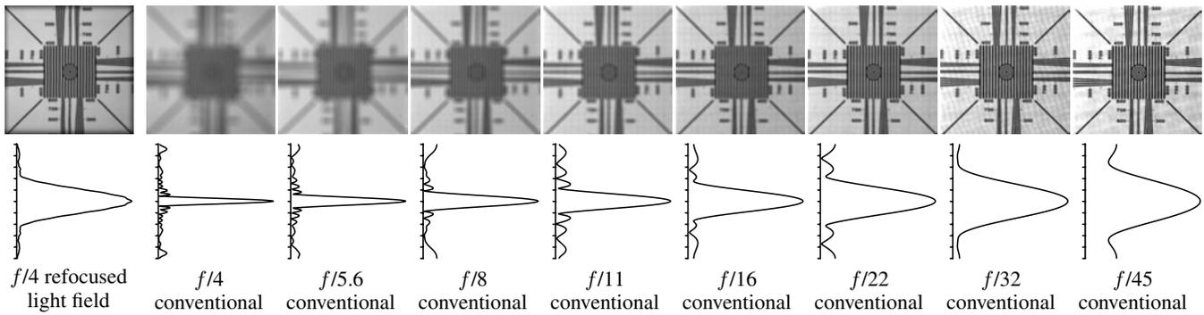
**Figure 10:** Top row shows photos of resolution chart. Bottom row plots (sideways, for easier comparison of widths) magnitude of center column of pixels in transfer function. Note that the  $f/4$  refocused light field best matches the conventional photo taken at  $f/22$ .
